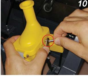
11 Unscrew the four splitter bracket fixing screws
